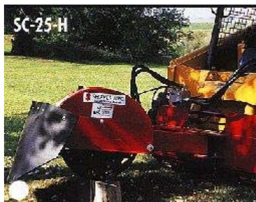
SC-25-H for 15 to 25 gpm Skid Steer Loaders
